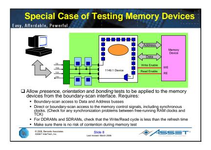
A boundary-scan (JTAG) interface can be used to test the *presence*, *orientation* and *bonding* of on-board RAM devices. The tests require JTAG (boundary-scan) access to the Data, Address and Control lines of the RAMs. Commercial PC-based test systems support this use of boundary-scan (JTAG) registers.
