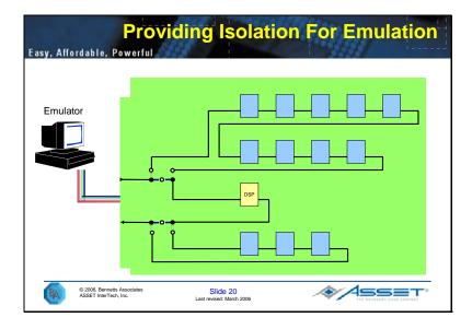
Most device emulators (DSP, RISC Emulators) have a problem unless their device is the only device in the scan chain. If these types of devices are placed in a full board-level boundary-scan (JTAG) chain, this can cause emulation-time and device isolation issues during development/software debug. It is better to provide an ability to isolate the emulation device entirely from the rest of the chain and so leave the other devices in functional mode to support the emulation process.
