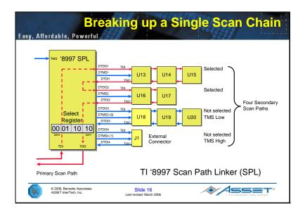
The slide shows a device from Texas Instruments called the '8997 Scan Path Linker (SPL). This device allows dynamic selection of secondary scan chains to be linked in with the primary scan chain. Such a device can be used to select, or otherwise, a subset of a main scan chain for a specific reason e.g. direct access to a flash device for programming purposes.
