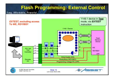
Flash Programming Set-up and Constraints
