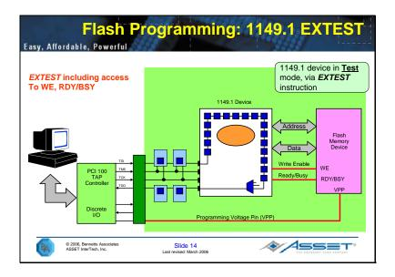
The next few slides takes a closer look at the ability to program flash memory devices through the boundary scan or JTAG registers of adjacent devices connected to the flash *Address* and *Data* pins.
