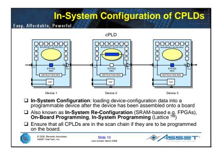
In-System Configuration (ISC), or In-System Programming (ISP) as it is often known, has become a major new application of 1149.1 boundary scan or JTAG. Basically, ISC is the ability to load configuration data into a Complex Programmable Logic Device (CPLD), Field-Programmable Gate Array (FPGA) or even a Flash device whilst such devices are mounted on a board.
