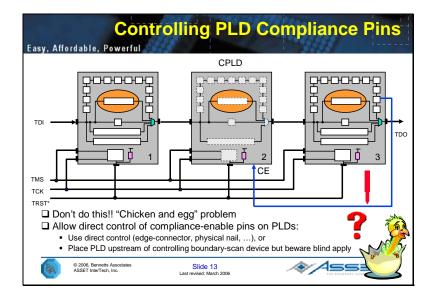
Do not place control of compliance-enable pins downstream of the programmable device. If you do this, the chain cannot be established – a classic chicken and egg problem. One solution is an automatic power-up reset circuit on the board that has control of the compliance-enable pins. Another solution is to place the programmable device downstream of the controlling device. (Note, this will not work if there is a defect that prevents the upstream devices from being correctly chained – see below.)
