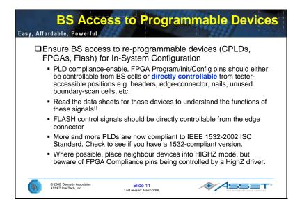
If the board contains programmable devices, such as CPLDs or FPGAs, make sure that the devices can be programmed, and re-programmed, from a boundary-scan/JTAG interface – see next slide. Ideally, such devices should be compliant to the new IEEE 1532 - 2002 In-System Configuration Standard.
