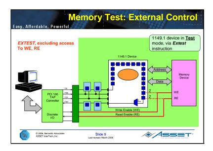
Here we see that the *WE* and *RE* control signals have been brought out to an edge-connector position to allow programmable IO pins (from the tester) to provide the control signals. This considerably reduces the time it takes to check the *presence*, *orientation* and *bonding* of the memory device.
