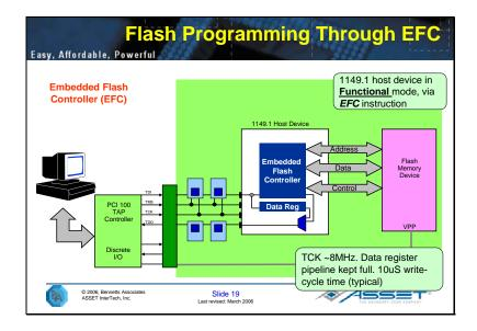
Another Solution: embed an Embedded Flash Controller (EFC) inside a host 1149.1 device, controlled via the device's 1149.1 structures. The host device TDI-TDO provides a path to an internal Data register to load the initial Address and Data. Once initialised, the embedded controller implements the programming procedure for the Flash, including all necessary control signals for Write and Read back. Incrementing the Address can be automatic.
