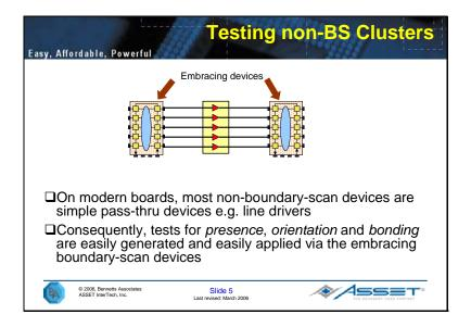
On most modern boards, the only non-boundary-scan devices are simple line drivers (buffers), with or without inversion, or re-routing devices such as multiplexers. These devices are generally known as "pass thru" devices. It is a simple matter to generate *Presence, Orientation* and *Bonding* tests for such devices and then apply the tests via the embracing JTAG or boundary-scan devices.
