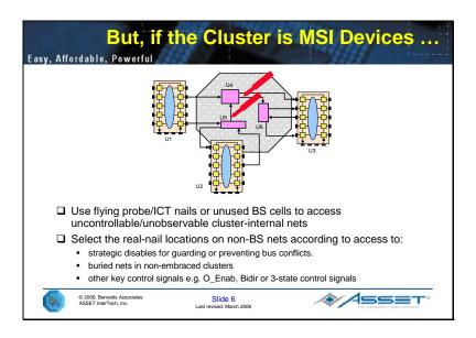
Testing non-BS MSI devices for opens and shorts via a JTAG (boundary-scan) interface (cluster testing) may not achieve 100% stuck-at and 2-net short fault coverage. Patterns for the non-boundary-scan clusters can be taken from the extensive libraries of In-Circuit Testers and validated via a fault simulator.
