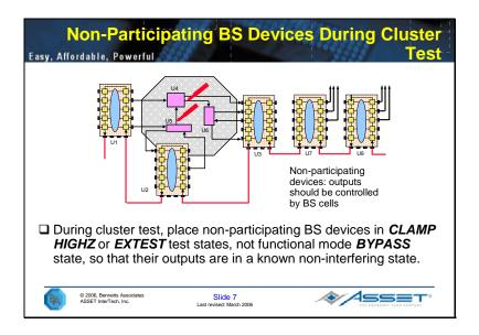
Boundary-scan/JTAG devices that do not participate in cluster testing should be placed into known safe states. One way to do this is to hold them in a test state rather than a functional state. The CLAMP, HIGHZ and EXTEST instructions can all be used to achieve this objective.
