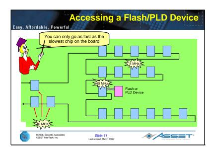
Here we see a Flash (or PLD) device accessible from an ASIC JTAG/boundary-scan device. Let us assume that we wish to program this device at the maximum rated frequency of 40MHz – the max TCK for the ASIC.
