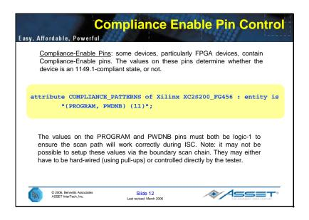
Xilinx xc2s200: an example of a programmable device that has compliance pins to establish the 1149.1 logic. The two pins, PROGRAM and PWDNB, must both be held at logic-1 to establish the boundary-scan logic.
